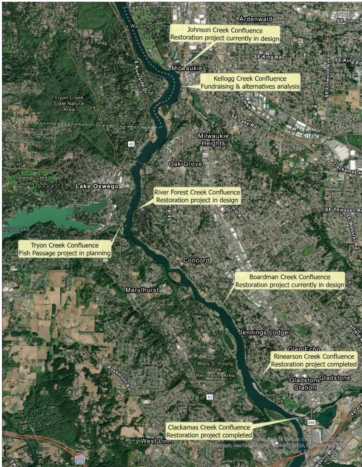
Figure 3 - Potential CWR along the lower Willamette River located in creek confluences.
