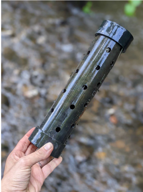
Figure 2 – All temperature loggers are protected in 2" ABS pipes that had 15-20 ¼ inch holes drilled out to allow water to through on a constant basis while preventing potential sediment accumulation around the probe.
